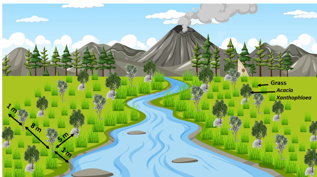
Figure 20. Example of a model for protection of riverbanks to preserve water quantity and quality
